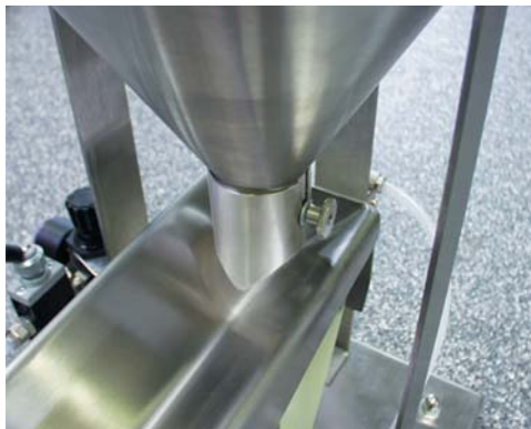
Dosing port at the silo outlet
