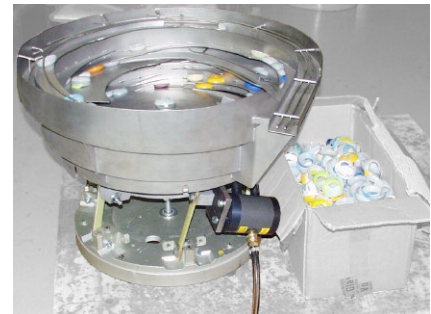
NTS 100/01 for spiral conveying of bulk materials
