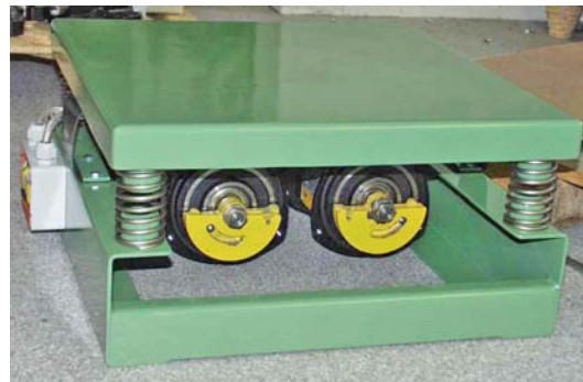
CC unbalances on 2 NEG's at vibrating table Coil springs made of stainless steel
