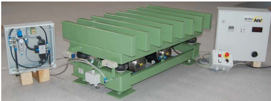
Maintenance unit, on/off switch and frequency control at the vibrating table
