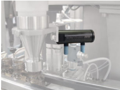
NTS 80 for filling small bottles
