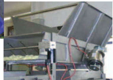
Conveying with stainless steel electric external vibrators
