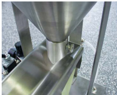
Dosing port at the silo outlet
