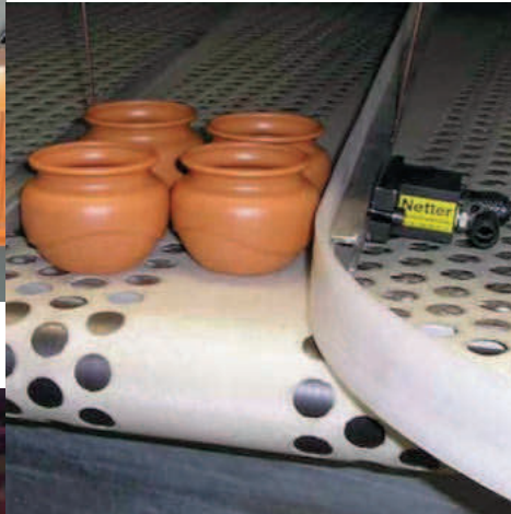
Avoiding product jams with pneumatic rotary vibrators
