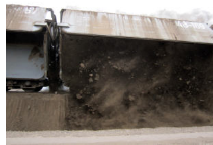
Cleaning from adhering ashes
