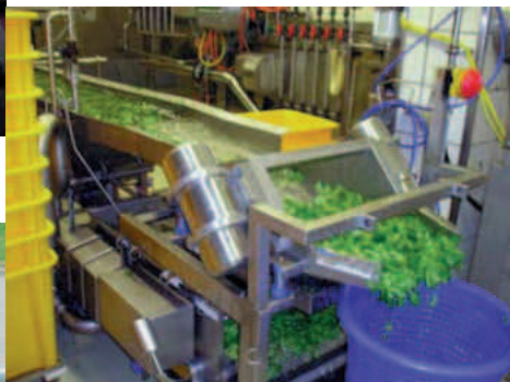
Conveyor sieving tray, driven by stainless steel electric external vibrators
