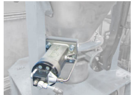
PKL 740 for loosening bridge formations
