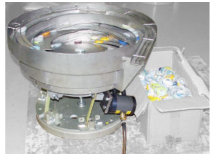
NTS 100/01 for spiral conveying of bulk materials
